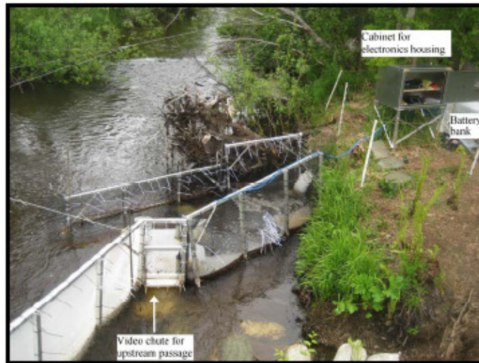
Photo 6. The downstream entrance to the underwater video chute, electronics housing, and battery bank at the weir on Stream 2002. The top of the photo is upstream.
